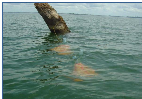
Figure 5: Set of Funnels Installed near Emerged Trunk
