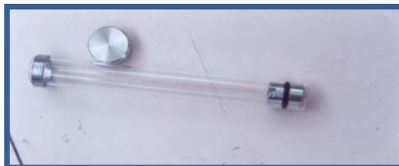
Figure 7: Gasometers to Transport the Samples to the Laboratory.
